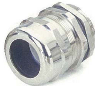
Nickle Plated Brass Gland - IP 68 - PG Thread
